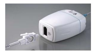
The Infinium *Capnotrac*® module is a field upgradable plug in module that can measure End-tidal Co<sub>2</sub> alone or End-tidal Co<sub>2</sub> with, O<sub>2</sub>, N<sub>2</sub>O, Halothane, Sevoflurane, Desflurane, Enflurane and Isoflorane gasses.
